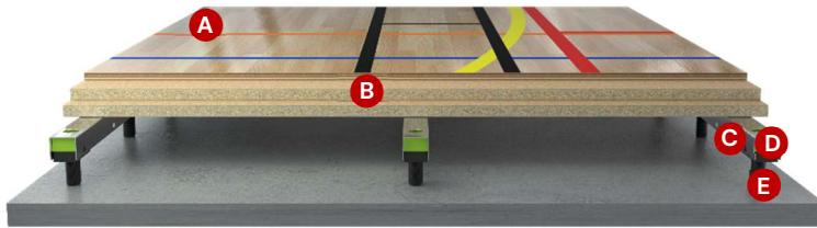
Adjustable height: 110–490 mm. Natural frequency = 23 Hz.
