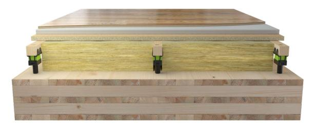
The standard distance between the girders is c/c 400mm to the second girder, then c/c 600mm, but this depends on the floor finish to be used. For example, for terrazzo, tiles and/or floating screed the distance between girders is c/c 300mm.
