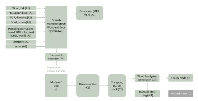
The wood subfloor system mainly consists of wood and in addition some polymer materials. The core process (A3) only uses energy in terms of electricity, and since the electricity production is accounted for in A3, there is no impact for A3 in the LCA model, except for the core waste. The core waste corresponds to minor waste flows such as plastics for recycling (MFR) and materials for energy recovery (MER) and here only a transport of the core waste has been considered.
